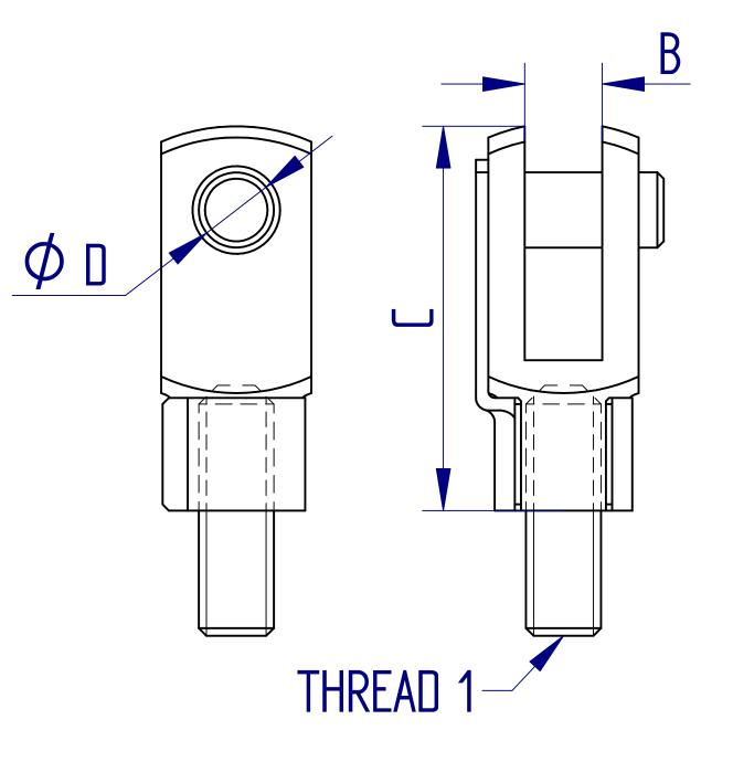
432-443 IS SUPPLIED WITH QUICK RELEASE CLEVIS PIN
