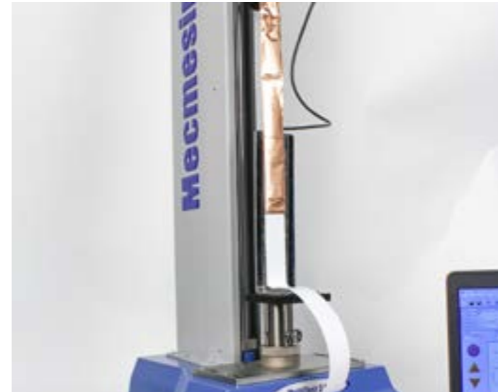
▲ Test Plate (PDV13016-C) shown with 50 mm strip being held in Upper Grip (Mec227-BG50)
