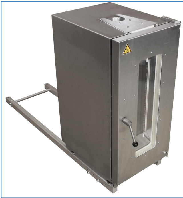
MEC2700 Retraction rails allow fore-aft movement of the cabinet into and out of the test space
