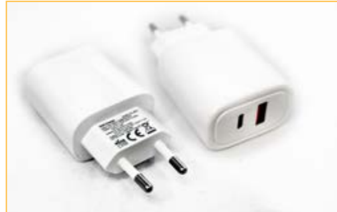
304-067, Europe, 2-pin round. Model CA-46AT, made in China input: 100-240V~50/60Hz 0.5A Output-C: 5.0V=3.0A; 9.0V=2.22A; 12.0V=1.5A Output-A: 3.6-6.5V=3.0A; 6.5-9.0V=2.0A; 9.0-12.0V=1.5A Output: A+C=20W Max
