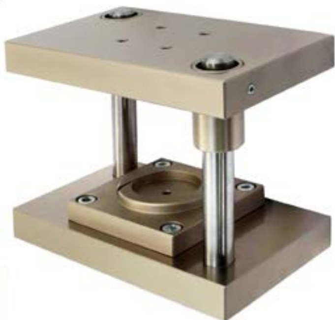
▼ PSV21062 Crush Test Fixture with Precision Guide. Ensures accurate alignment during compression to facilitate testing to ISO3037, ISO12192, TAPPI T822 and T811. May be combined with ECT, FCT and RCT fixtures (order separately). Shown here with RCT lower carrier.
