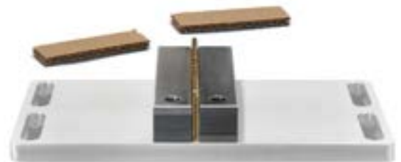
▲ PDV14137 Edge Crush Test Guide Blocks shown attached to PDV11089 Anvil Plate with rectangular fibreboard test pieces.
