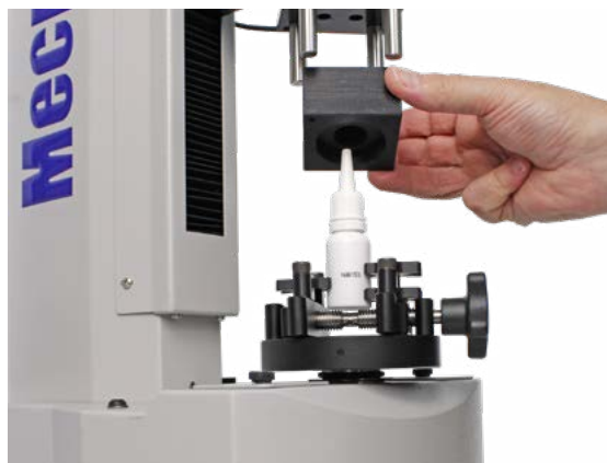
Lower Precision Fixing Table (Helixa) shown with V-jaws fitted. Part nos: 432-600 and 432-602 (photo is helixa-bottle-mandrel.png)
