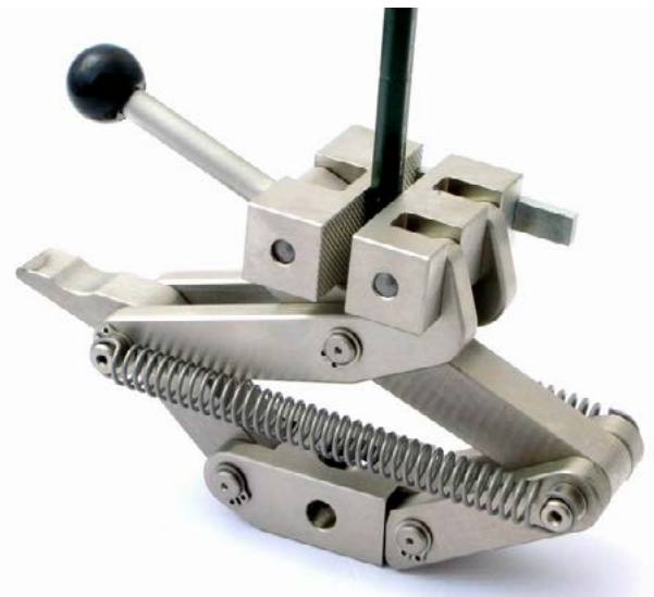
Mec11-5 with Mec11-5-BP pyramid jaws
