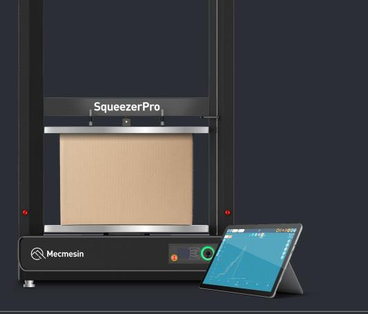
Crafted to evaluate box performance, SqueezerPro offers powerful insights into the compressive strength performance of various board mediums, closures, interior partitions, and other critical design variables. Additionally, SqueezerPro can be used to conduct distribution simulation compression testing for individual packages.
