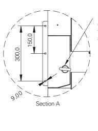
M16 eye bolt, can be removed to provide a M16 anchor point
