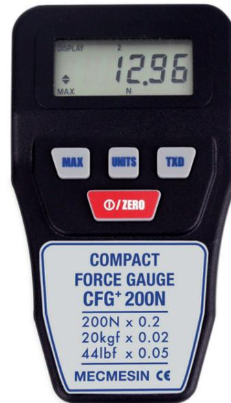
Peak readings captured at 500 Hz with an accuracy of  $\pm 0.5\%$  of full scale
