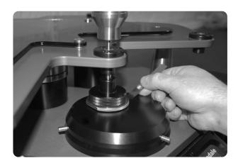
The James Heal Martindale calibration service offers a comprehensive check into 12 different points on the instrument, ensuring it complies with strict measurements as set by UKAS. These include abrasion and pilling lissajous figures, spindle bearing friction, sample holder insert protrusion and the parallelism between the abrading table and sample holder insert.
