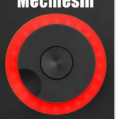
Lights indicate stand status Dial positions drive spindle precisely Centre button confirms menu settings
