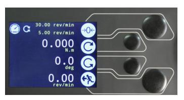
Clear colour display of status, clockwise and anticlockwise speeds, position and torque.
