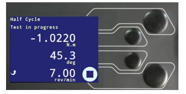
Continuous live readings during testing, including status and cycle count, plus peak and break capture by AFTI, or full data capture and plotting with VectorPro™ Lite.
