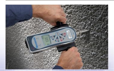
Mecmesin's shotcrete penetrometer provides accurate readings of the forces required to penetrate sprayed or poured concrete during the first few hours of development, giving a reliable indication of compressive strength. Its accuracy and portability make it ideal for on-site testing to BS EN ISO 14488 (Method A) and related standards.
