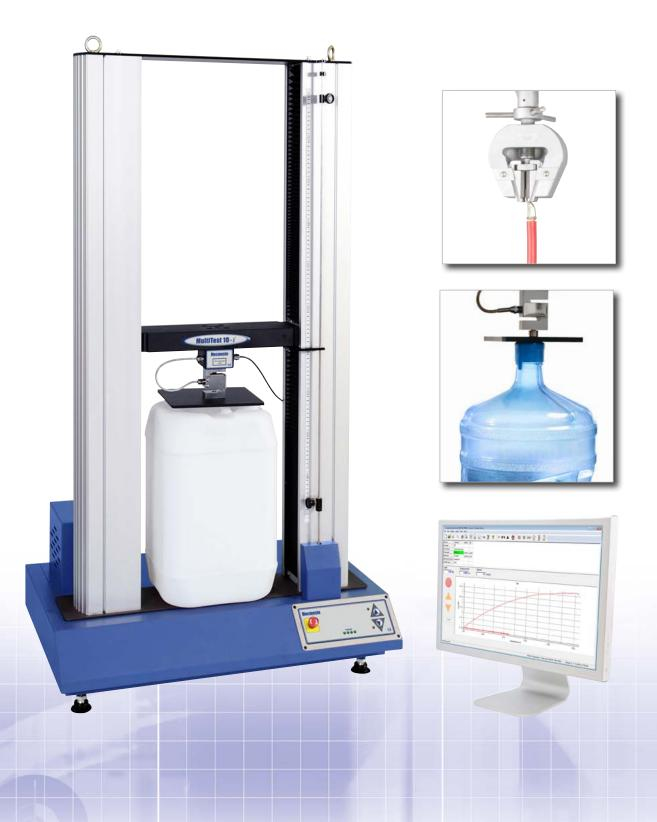
The Mecmesin MultiTest-*i* range of test frames sets the standard in computer-controlled testing, operating through the power of Emperor<sup>TM</sup>; easy-to-use yet powerful force testing and analysis software.
